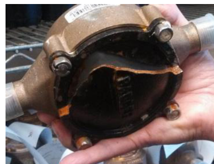
Broken Water Meter, Madison Water Utility: January 8, 2014
